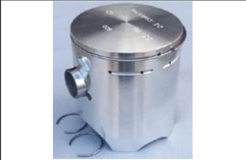
3960 Piston Di Carmine 53,96 piston pin is 24 mm. from top
